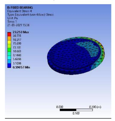
Equivalent stress on the concrete: -
