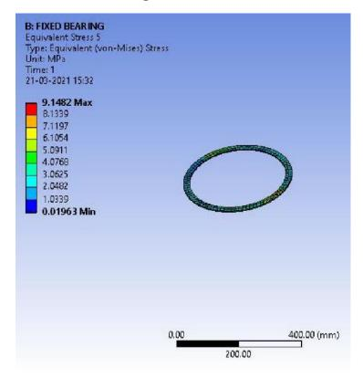
Equivalent stress on the elastomeric pad: -
